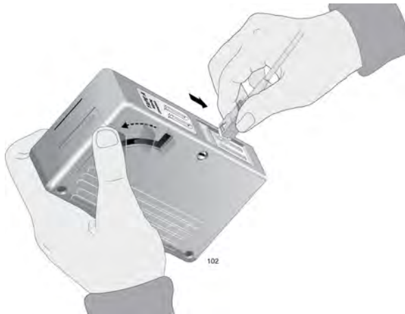
Figure 23. Rubbing the Ferrule Tip on the Cleaning Surface
