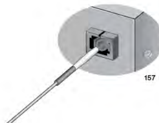
Figure 25. Cleaning a Recessed Ferrule
