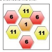
**Figure 4 Microcell WLAN**
