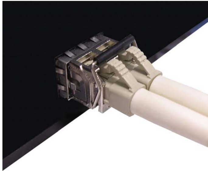
LC connector to the transceiver
