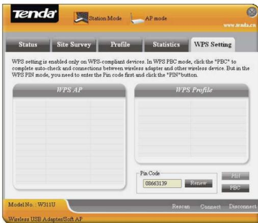
**PIN:** Enter the Pin code and click the “PIN” to automatically connect the wireless adapter with wireless devices around.
