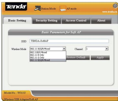
**SSID:** Wireless network's ID name scanned by wireless adapter.
