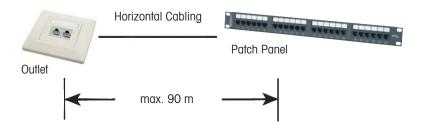
**Channel**—the connection from an active device (e.g. a switch) in a data rack to a network card, patch cords included. The recommended maximum length of equipment cords in data racks is 5 m; the maximum recommended length for work area cords is 20 m. The length of the channel (i.e. the horizontal cabling plus an equipment cord as well as a work-area cord) should not exceed 100 m.
