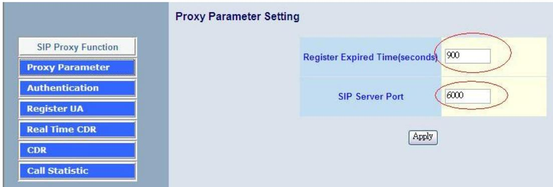
Setp\_3: In Proxy Parameter setting, You can set SVR Port and registered time. For example, in this setting Port is 6000 and registered Expired 900 second. Default Proxy port is 5060.
