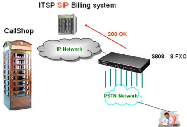
The gateway can send the “200 BYE” SIP signals to Billing System of ITSP, after the user hang up the Phone and detect PSTN line disconnect voltage.
