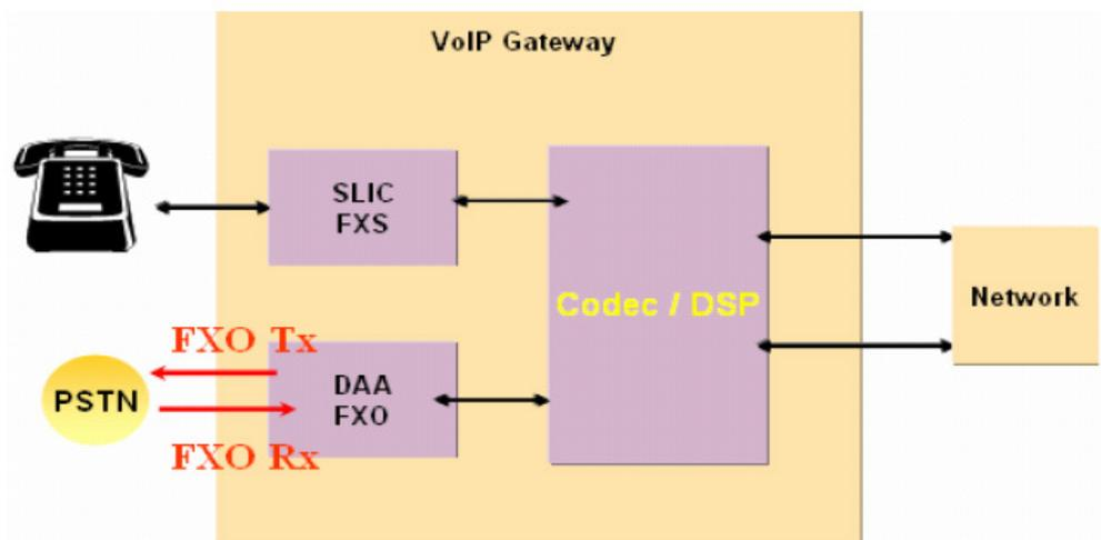
Supports multiple levels of gain and attenuation for the transmit and receive paths of DAA.
