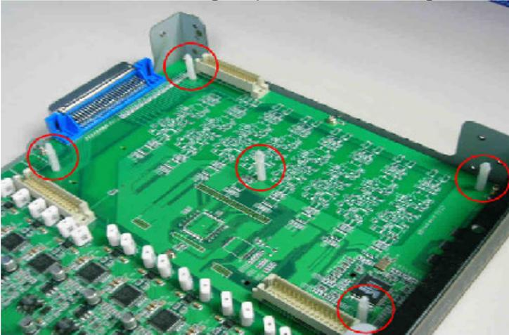
e.) Put and fix the module board on motherboard. Please notice the triangular mark on module and motherboard is on the same position. Please fix DIN41612 connector is regular and good, at the same time the regular post totally opens and blocks the module too.
