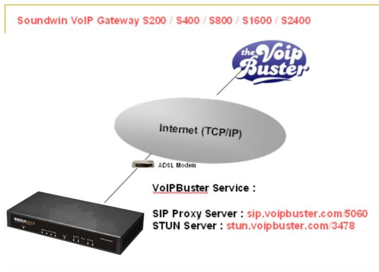
The 065-9200S/400S/S800/065-9800S/1600S/2400S VoIP Gateway can register to VoIPBuster (<http://www.voipbuster.com>) VoIP service by SIP protocol and also can call SIP calls by VoIPbuster (<http://www.voipbuster.com>) service.
