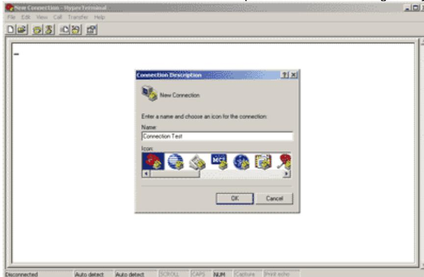
5. Make connection(Bits Pre second:**38400** Flow control: **None**)
