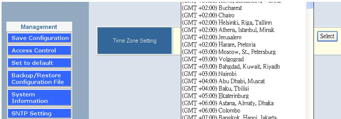
**Use SNTP Setting**—When checked, Gateway uses a Simple Network Time Protocol (SNTP) to set the date and time . The Gateway synchronizes the Gateway’s time after you select the time zone. *Use SNTP Setting*, Select the time zone which Gateway was at.
