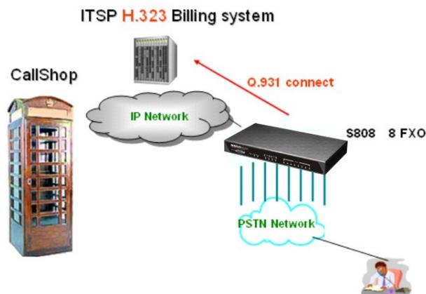
The gateway can send the “Q.931 Release” H.323 signals to Billing System of ITSP, after the user hang up the Phone and detect PSTN line disconnect voltage.
