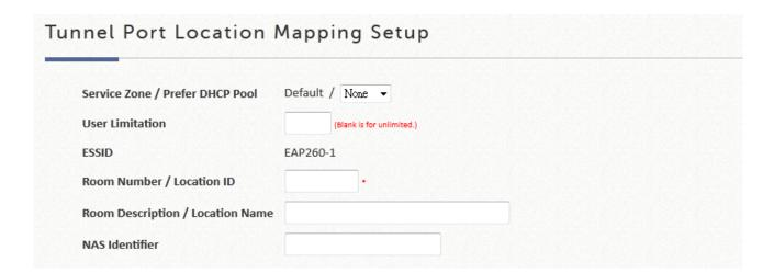
Once the VAP tunneled back, complete tunnel or split tunnel, has been configured with PLM (Port Location Mapping), remote sites may also benefit from the PMS system or other centrally managed hotspot operations which require location attributes or information.
