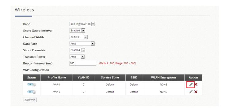
The SSID and Wireless Security can be specified per Service Zone. Depending on deployment needs, access filtering may be imposed on individual Service Zone's managed AP devices. The Wireless Settings section under the VAP Configuration list allows the specification of wireless settings including Access Control list.
