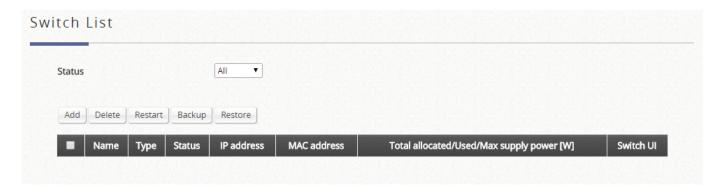
The Switch's name will be shown as a hyperlink. Click the hyperlink of each managed SW1024 for further configuration (General Setting, PoE Setting, VLAN Membership Setting, Port Setting, Poe Schedule) on the switch.
