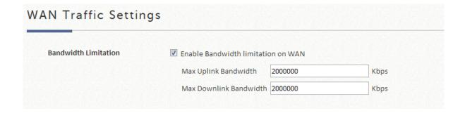
The Uplink and Downlink bandwidth configured here is the combined bandwidth for WAN interface including WAN1 and WAN2. However, please note that the actual bandwidth is still bounded by the network speed of your ISP operator. For instance, when the network speed of your ISP is limited to 1Gbps, the total throughput under such constraint will not be greater than 1Gbps even if you configure 2Gbps on the Controller.
