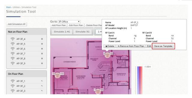
Simulation can be done by clicking the *Simulate 2.4G* or the *Simulate 5G* button. If the results are satisfactory, the settings on each AP may be saved as a template to be used to apply to APs in AP Management.
