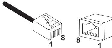
Figure 16. RJ-45 Connector and Port Pin Layout
