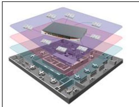
**Figure 3 Channel Blanket Deployment**
