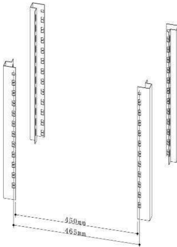
Center distance of the horizontal installation hole and net horizontal installation space
