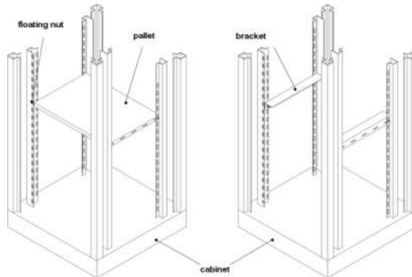
Check whether the floating nut for fixing the device is installed in the square hole of the cabinet column. If not, insert the floating nut to the square hole according to the position of the pallet or tray.
